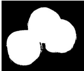
Fig. 10. The result of colouring black areas of objects using contour search
