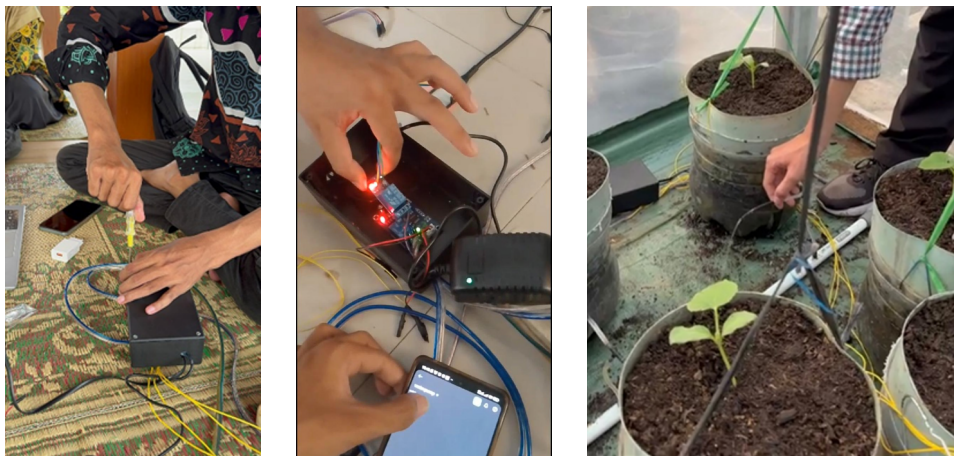
Fig. 4. Wiring, programming, and system testing of automated plant watering
