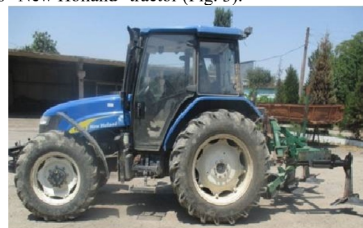
Fig. 3. UK-3 vine cultivator integrated into the TL-100 "New Holland" tractor.
