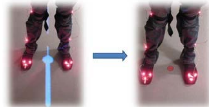
Fig. 7: video-projected line indicating the start position and orientation (left) and target position with implicit target orientation (right).
