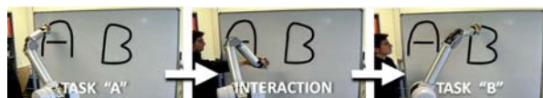
Figure 4: Bilateral human-robot interaction in which the robot is used by the user as a tangible interface to start/resume tasks and switch between tasks. The robot is gravity-compensated and can be moved without effort. When the user brings the robot in a known region in which a task has previously been demonstrated, the robot recognizes this part of the movement and continues the task actively until the user decides to stop it by physically moving it away from the task, or possibly bringing it towards another task region. See [6] for details.
