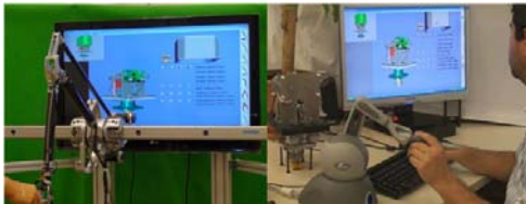
Figure 1. IMA-VR Training Platform: the trainee interacts and manipulates the virtual scene combining haptic, audio and visual feedback. The platform can be used with different types of haptic devices such as desktop workspace (right) and large workspace (left).
