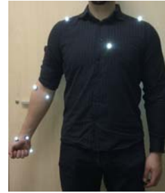
Figure 3: Configuration of markers adopted to recognize the seven degrees of freedom of the right arm. The three markers on the chest provides a reference for shoulder angles.
