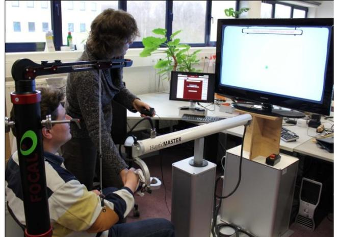
**Figure 1: Hardware Setup, including haptic master, sling and visual display**
