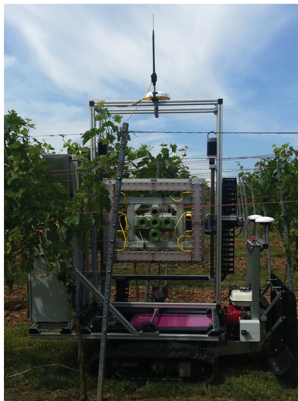
Figure 1. PHENObot is a system for rapid data acquisition along with a GPS track. Currently the system works image based but extension for further sensors is anticipated.
