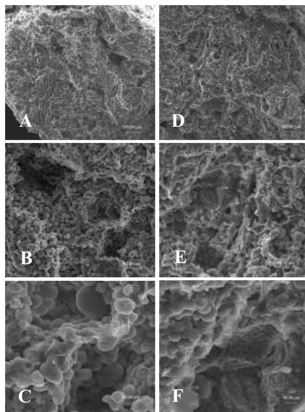
**Fig. 6.** Cross-section with various magnifications of control CFBS pasta (A x 200, B x 600, C x 1500) and optimum pasta with the addition of HTCF (D x 200, E x 600, F x 1500) observed with SEM.
