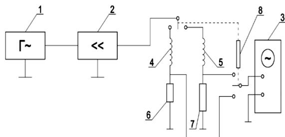
1 – generator; 2 – amplifier; 3 – oscilloscope; 4 – solenoid 1 (large); 5 – solenoid 2 (small); 6 – solenoid current control resistor 1 (1 Ohm); 7 – solenoid current control resistor 2 (4 Ohm); 8 – solenoid select switch
