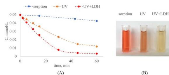
Fig. 2. (A) Kinetic curve of adsorption of Congo red dye on Mg/AlNi - LDH and kinetic curves of photodegradation of Congo red dye in the presence of LDH and without it; (B) Images of residual dye solutions after adsorption and after photodegradation during 60 min.
