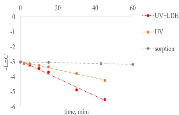
**Fig. 3.** Pseudo-first-order kinetic plotting of adsorption data and photodegradation.
