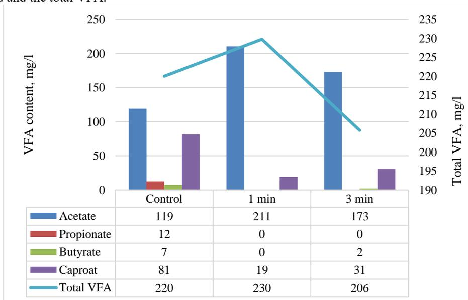
**Fig. 5.** The content of volatile fatty acids in the confectionery wastewater after 1 and 3 min of pretreatment in VLA, and control - without pretreatment in VLA.
