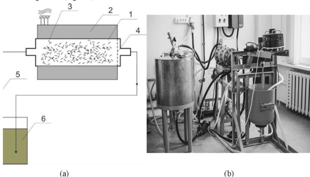
**Fig. 1.** Schematic diagram (a) and general view (b) of the vortex layer apparatus: 1 - chamber made of non-magnetic material; 2 - inductor that creates a rotating magnetic field; 3 - ferromagnetic particles; 4 - grid; 5 - pump; 6 - container with a substrate.
