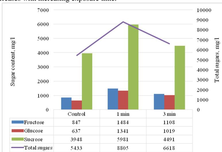
**Fig. 4.** Content of sugars in wastewater of confectionery production before and after treatment in VLA.
