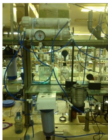
Fig. 2. Water quality assurance unit: schematic diagram (a) and photo (b). 1 – ion-exchange filter 2, 3 – reverse osmosis apparatus.
