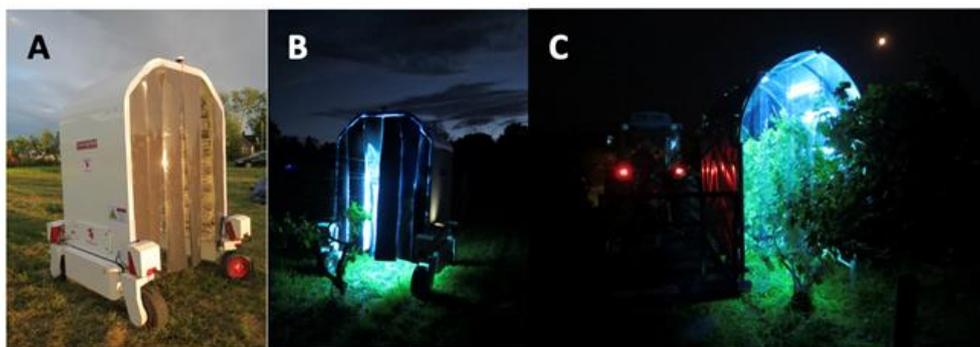
Figure 1: UV lamp arrays used for nighttime applications in vineyards were either carried by an autonomous robotic carriage (A and B), or were tractor-drawn (C)
