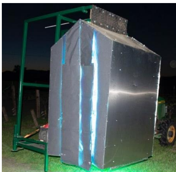
Figure 2: The tractor mounted vineyard UVC application unit in operation at night.
