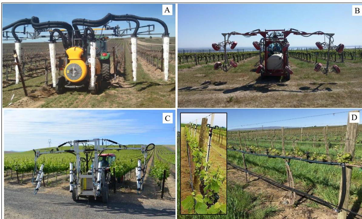
Figure 3: Vineyard sprayers assessed for deposition in Washington, USA vineyards. Three machines—(A) Gregoire, (B) Quantum Mist, and (C) On Target—are commercially available. The (D) Solid Set Canopy Delivery System (SSCDS) is a proof-of-concept fixed spray system installed with disc-core nozzles along the drip irrigation and a separate emitter in the canopy.
