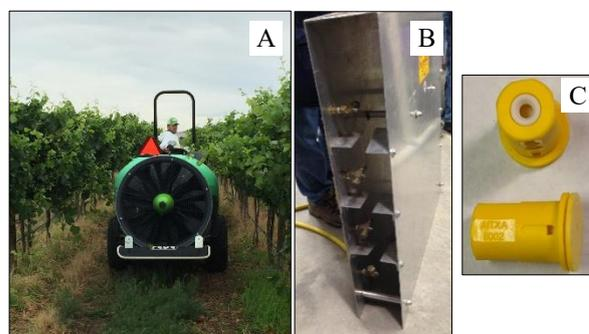
Figure 2: (a) Axial-fan air-blast sprayer with nozzle bodies surrounding the larger single fan, (b) example of a small
