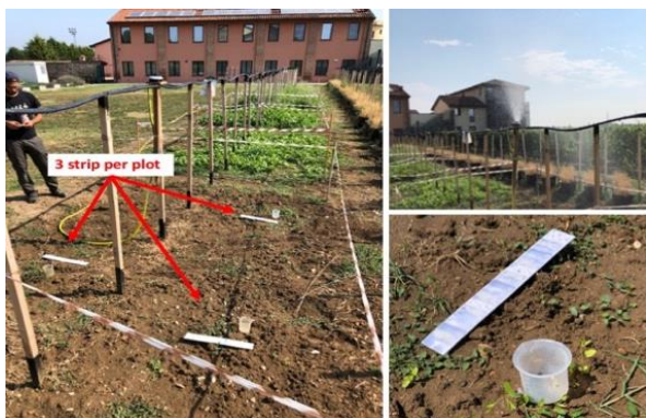
Figure 2. Rain simulation-splash experiment: blotted-paper strips posed on the ground of each plot allowed to quantify the interference of the cover crop with simulated rainfall
