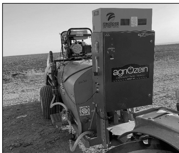
Figure 2: The OWS system consisted of a commercially available generator, injector and recirculating pump (AgriOzien, Nebraska, USA) retrofitted to a Rears Manufacturing Powerblast Pul-Tank airblast Sprayer (Oregon, USA), by Washington State University - Center for Precision and Automated Agricultural Systems.
