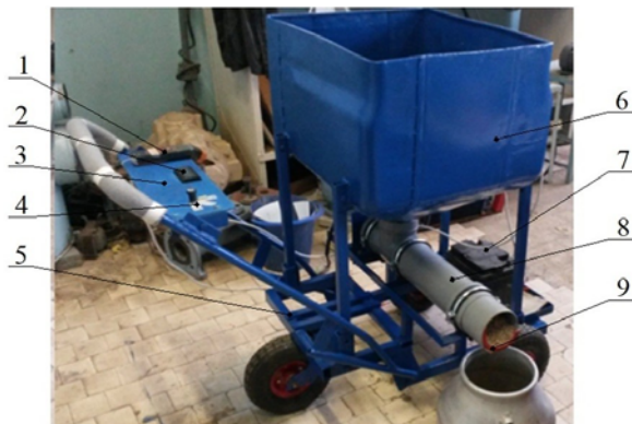
Fig. 1. Mobile fodder dispenser with a spiral-screwed dosing unit: 1 – SM8238 turn counter, 2 – MYLB-G.T. Power RC 130A measuring system, 3 – control panel, 4 – mode switch, 5 – handcart, 6 – tanker for concentrated fodder, 7 – battery, 8 – tubular enclosure, 9 – spiral.
