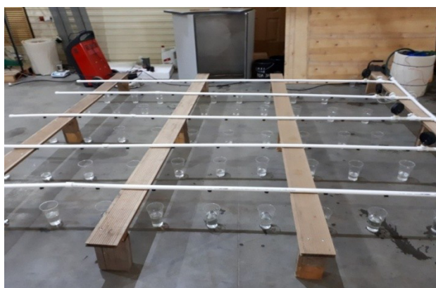
Fig. 8. Experimental installation for drip irrigation.
