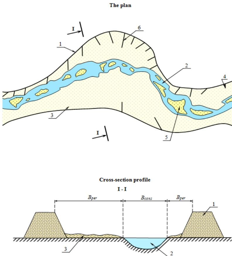
**Fig. 1.** The plan and cross-section profile regulated a site of bed of the river Amu Darya. 1- longitudinal dam; 2- constantly working part of a channel; 3- periodically working part of a bed; 4- spur; 5- island; 6- cross-section dam.
