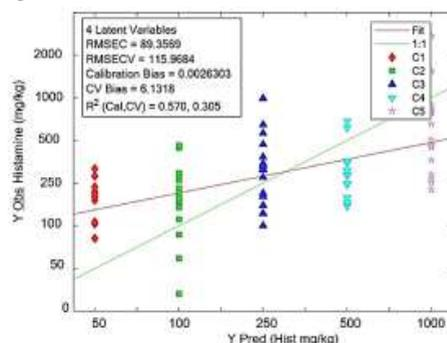
**Fig. 2.** NIR predicted vs observed histamine levels in the regression model of Whatman 2 samples. Concentrations are: C1 - 0.5 mg/kg; C2 - 1 mg/kg; C3 - 2.5 mg/kg; C4 - 5 mg/kg; C5 - 10 mg/kg
