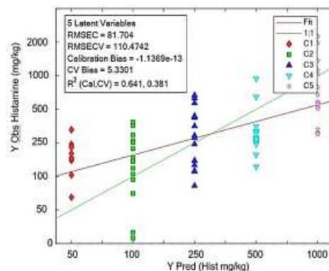
**Fig. 3.** NIR predicted vs observed histamine levels in the regression model of Whatman 2 samples. Concentrations are: C1 - 0.5 mg/kg; C2 - 1 mg/kg; C3 - 2.5 mg/kg; C4 - 5 mg/kg; C5 - 10 mg/kg
