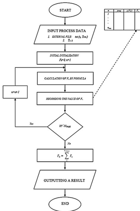
Fig. 4. Block diagram of a web-based calculator for calculating the *F effect*
