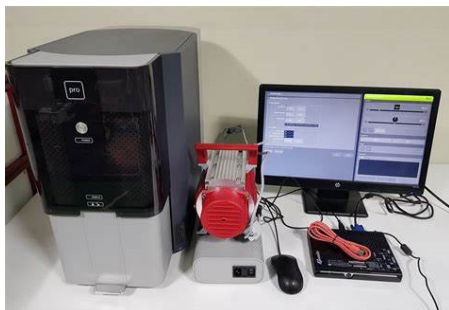
Figure 2: The schematic diagram of scanning electron microscope
