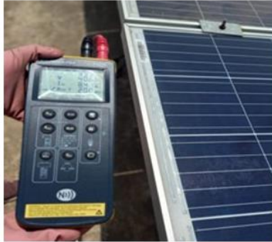
Figure .1. Solar I-V Curve tracer connected to actual PV system under field conditions.
