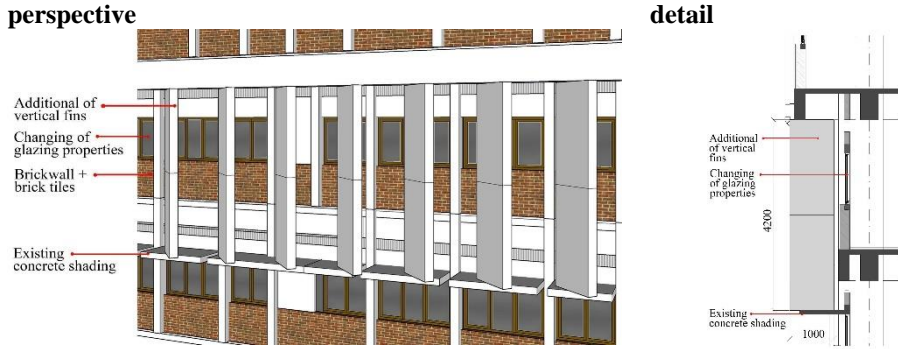
Fig. 6. Combination of Vertical Fins and Changing the Glazing Properties Source: Author's documentations
