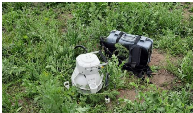
Fig. 8. LI-COR - 7810 mobile gas analyzer on a carbon farm
