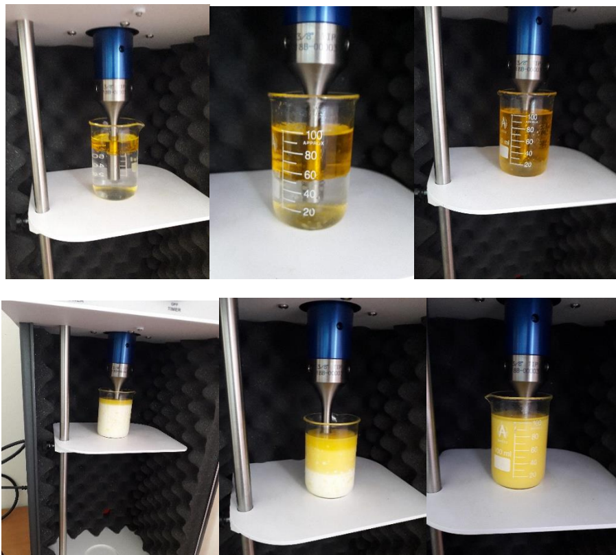
Fig.2. Ultrasonic treatment of a water-oil composition based on safflower oil.
