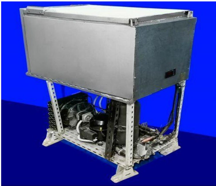
Fig. 2. Low-temperature refrigerating chest with a mixture of refrigerants with sequential condensation of components
