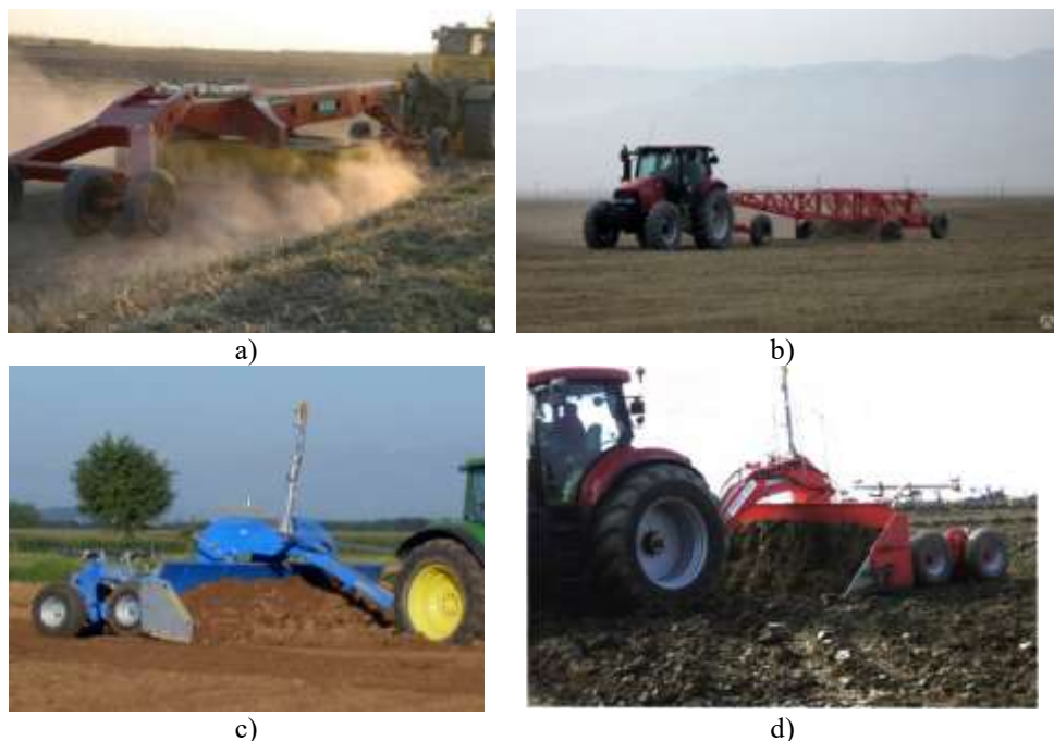
Fig. 3. Levellers for leveling fields: a) long base D-719; b) trailer P-2.8; c) scraper SP-4.2; d) scraper "Kholmogor 3700".
