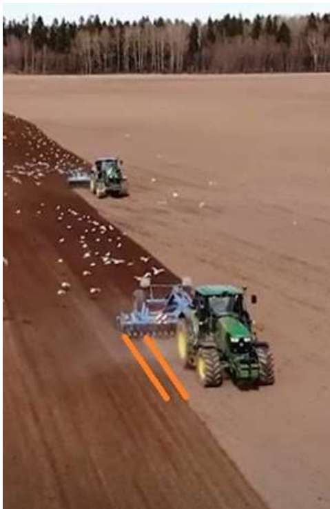
Fig. 1. Area treated twice with JD 6195M + Lemken Rubin 500 KAU aggregates.
