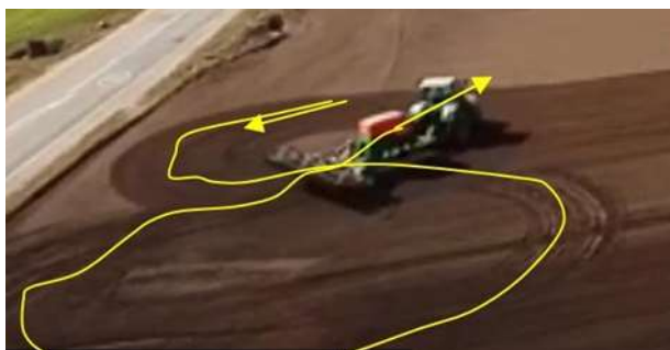
Fig. 6. The scheme of turning at the end of the rut using the "figure eight" reception with manual control.
