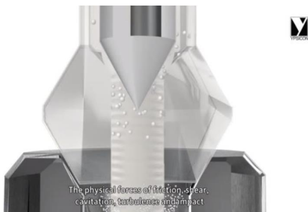
Figure 1. UHPH valve and nanofragmentation effect ( https://www.ypsicon.com/ ).
