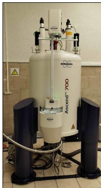
Figure 2. Magnet unit of the BRUKER NMR spectrometer Avance™ NEO 700.
