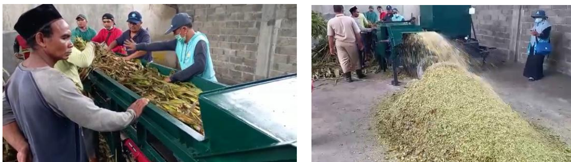
Fig. 7. The performance test of the Cross Flow type Sorghum Chopper
