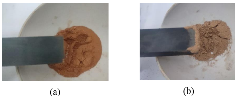
Figure 1. The synthesized MIL-100(Fe) (a), and MIL-100(Fe) @Fe_3O_4 (b) were exposed to an external magnetic field
