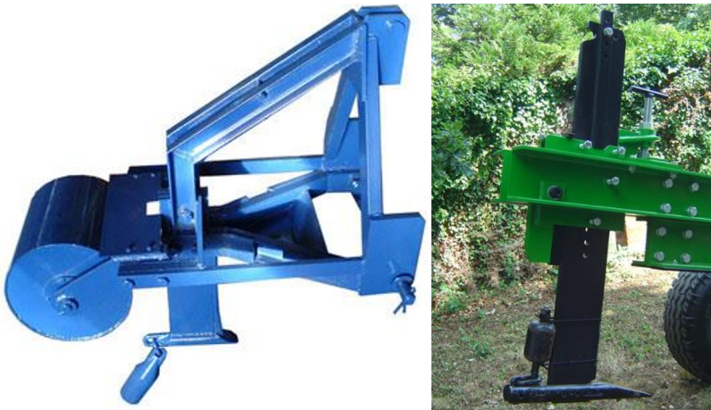
Fig. 8. A mole rat with a "Yugagromash" stand (left) and a "Miles Drainage" stand (right).
