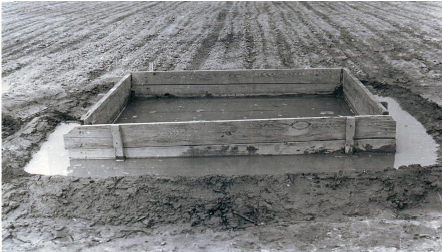
Fig. 2. Determining the field moisture capacity of the soil by the square frame method.
