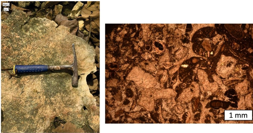
Fig. 4. Appearance of limestone with Clastic facies Packstone LP 7 (left) and thin section of Packstone limestone (right)
