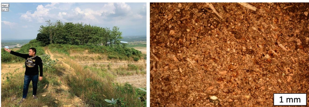
Fig. 5. Appearance of limestone with Clastic facies Packstone LP 10 (left) and thin section of Packstone limestone (right)
