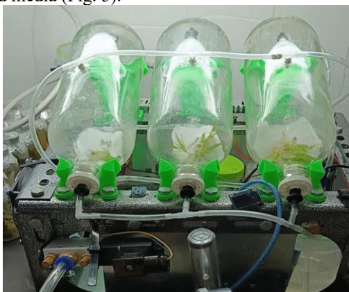
Fig. 5. Application Micropropagation C. pandurata in Temporary Immersion Bioreactor Systems.
