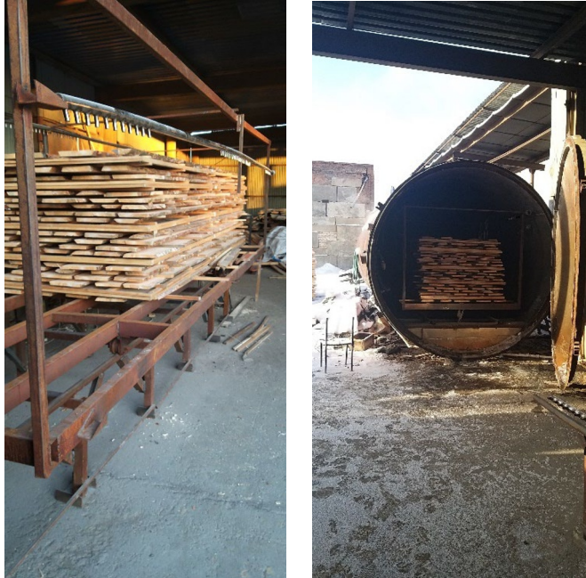
Fig. 3. Loading lumber into a vacuum chamber with installed film electric heaters.
