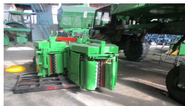
Fig. 2. Two-row harvesting apparatus for intensive processing of cotton boxes (IPCB) with row spacing 76 cm, prepared for attachment to the machine CHM-3.04H.
