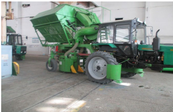
Fig. 3. Semi-mounted cotton harvesting machine CHM-1,8 based on the tractor MTF-80 "Belarus", equipped with a harvesting apparatus for IPCB-№1, manufactured under project №T-KX-2021-176.
