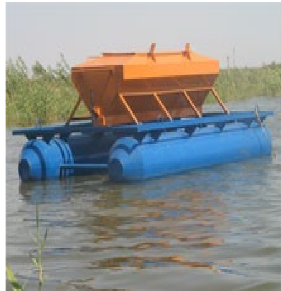
Fig 2. Multi pendulum auto-feeder "Reflex-T 1000-16".
