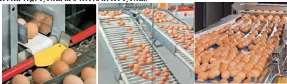
Fig. 4. Eggs transfer from cage system into cross belt (left); eggs during rod conveyors (middle); and final eggs collection results (right) [5].
