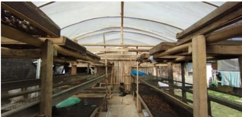
Fig. 1. A simple solar dryer with a layer of clear plastic roof in which a natural convection air flow takes place.
