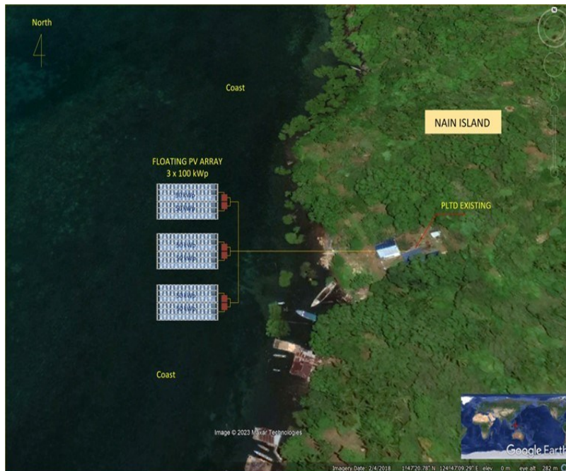
Fig. 8. Layout of the proposed hybrid FPV-diesel power plant.
