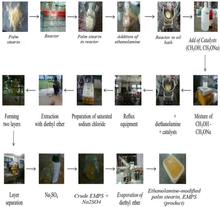
Fig. 2. The flow diagram of the preparation of EMPS
