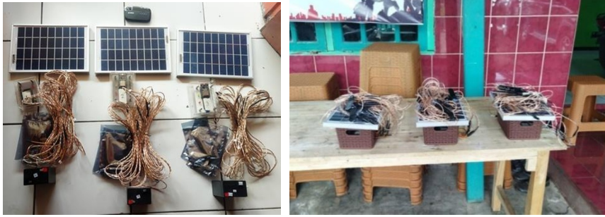
Fig. 6. ApparApearance of soil moisture monitorings system based on IoT ESP32.
