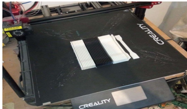
Fig. 3. The 3D printing method was used to manufacture polymer tensile test samples
