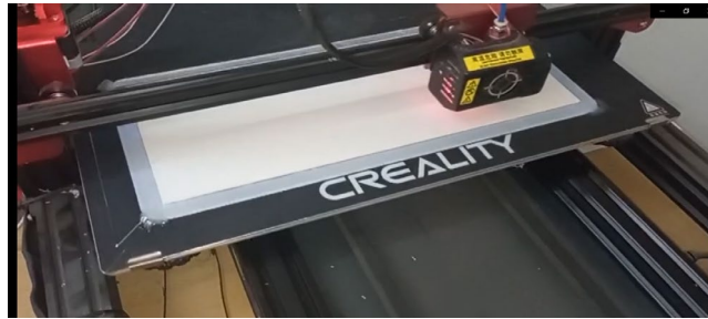
Fig. 6. Manufacturing FG specimens using 3-D printing
