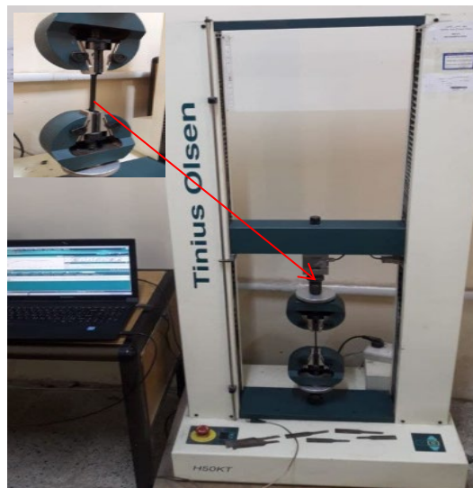
Fig. 3. The 3D printing method was used to manufacture polymer tensile test samples
