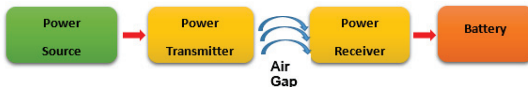
Fig. 2. Basic Structure of Wireless Charging System
